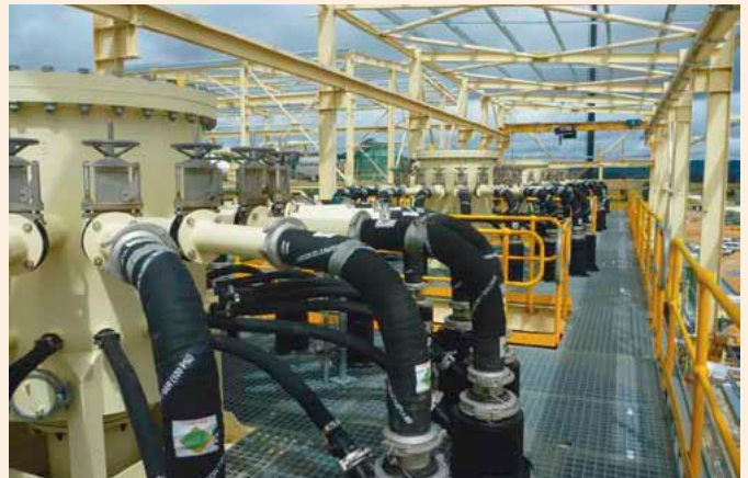
Moorlaben Coal Mines using 2 stage flotation with 4 x B6000/20 Jameson Cells (NSW, Australia)
